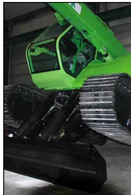
VBLADE leveling enables working on slopes up to 19° (34%)
