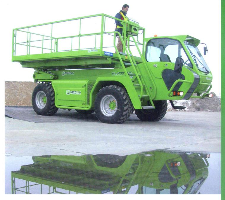
The operator can control any movement with the proportional controls available in the platform, including machine travel (with automatic maximum speed limiter) and the all-wheel steering. Driven from the platform, maximum speed is 6 kph with the boom stowed, and 1 kph with the boom raised to the full working height.
