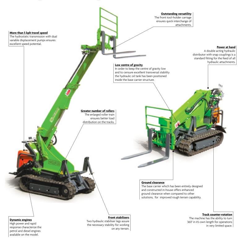
The Cingo M10 with Handler 200 attachment provides a sturdy and reliable machine. The telescopic boom can be fitted with various attachments (buckets, forks, clamps, and skips) to carry out different kinds of tasks.
