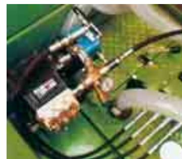
A high pressure machine washing pump, essential for the long life operation of vehicle, drum and tank.
