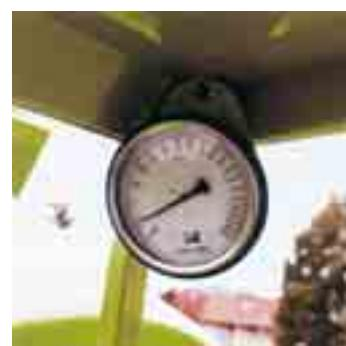
Provides material weighing to an accuracy of 8% of the indicated figure.
